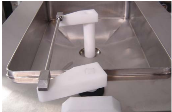
Figure 3-2 Flow Control Assembly
