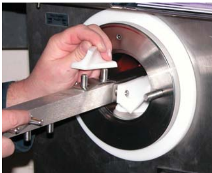
Figure 3-5 Installing Auger Blades
